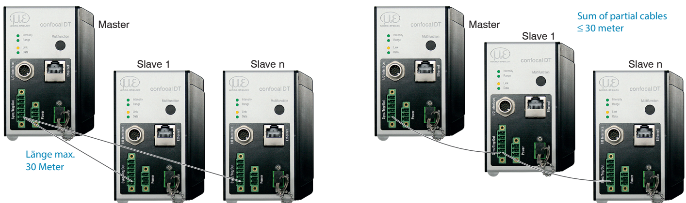
Fig. 17 Synchronization of multiple controllers, star-shaped on the left, daisy-chained on the right
