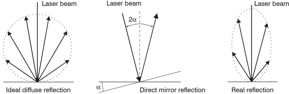
Abb. 3 Reflectance of target surface
