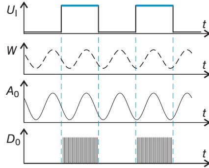
Abb. 22 High trigger level (top) with analog output  $A_0$  and RS422 output signal  $D_0$  (bottom)
