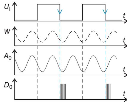
Abb. 23 HL trigger edge (top) with analog output  $A_0$  and RS422 output signal  $D_0$  (bottom)
