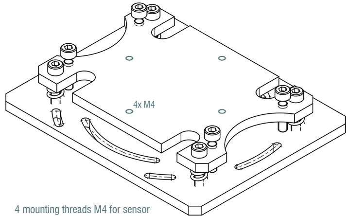
4 mounting threads M4 for sensor mounting, optional: sensor rotated by 90°.
