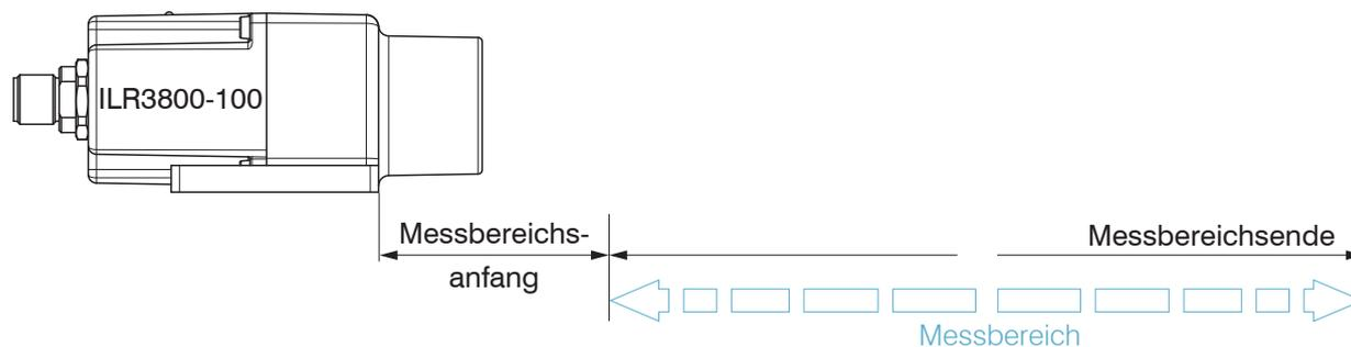
Abb. 8 Housing edge as point of reference for start of measuring range
