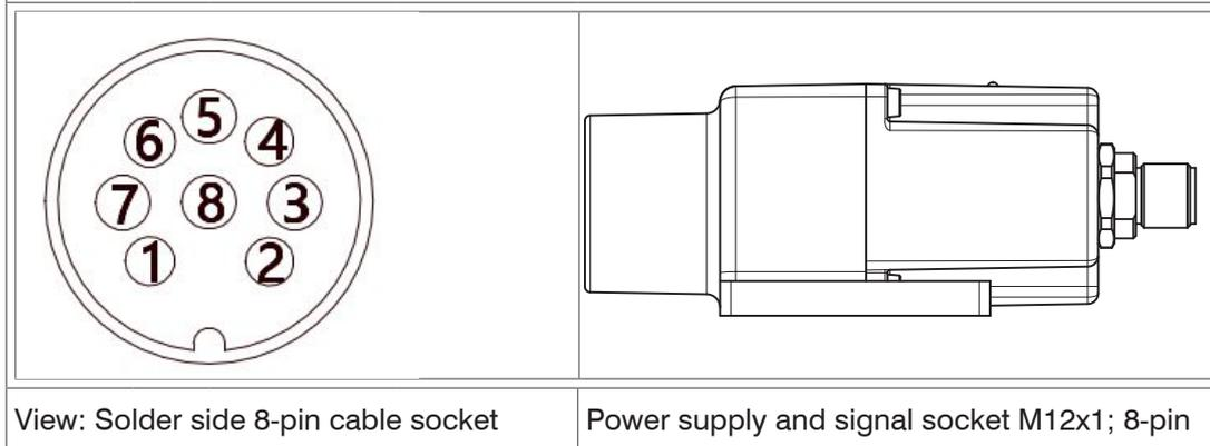
View: Solder side 8-pin cable socket
