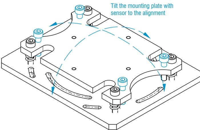
Tilt the mounting plate with sensor to the alignment
