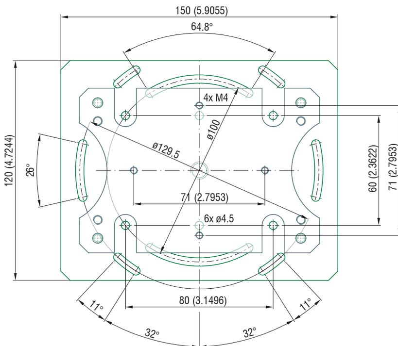
Abb. 32 Dimensional drawing mounting plate ILR-MP3800, dimensions in mm (inches, rounded off)
