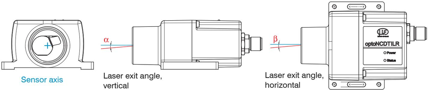
Abb. 9 Manufacturing tolerance laser exit versus sensor axis
