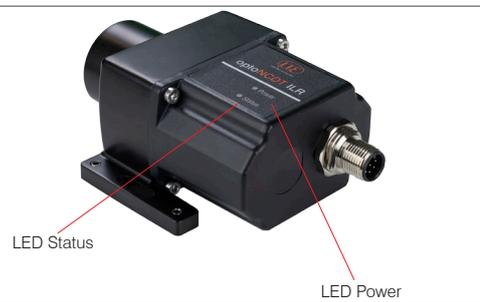
The Signal LED indicates the reflection strength of a measurement. This LED generally lights up when a measurement is started. If the Power indicator turns red and the Status indicator turns yellow at the same time, a boot error has occurred. Recovery is necessary.
