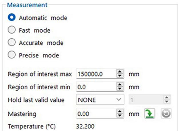
Abb. 19 Data acquisition menu, for selecting measurement mode, etc.
