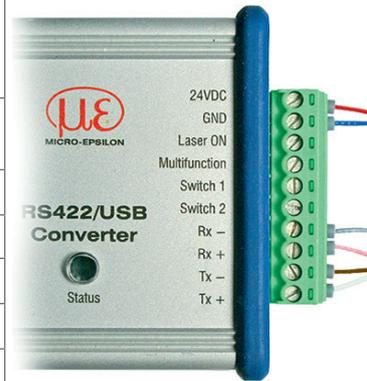
Symmetrical differential signals according to EIA-422, not electrically separated from the voltage supply.
