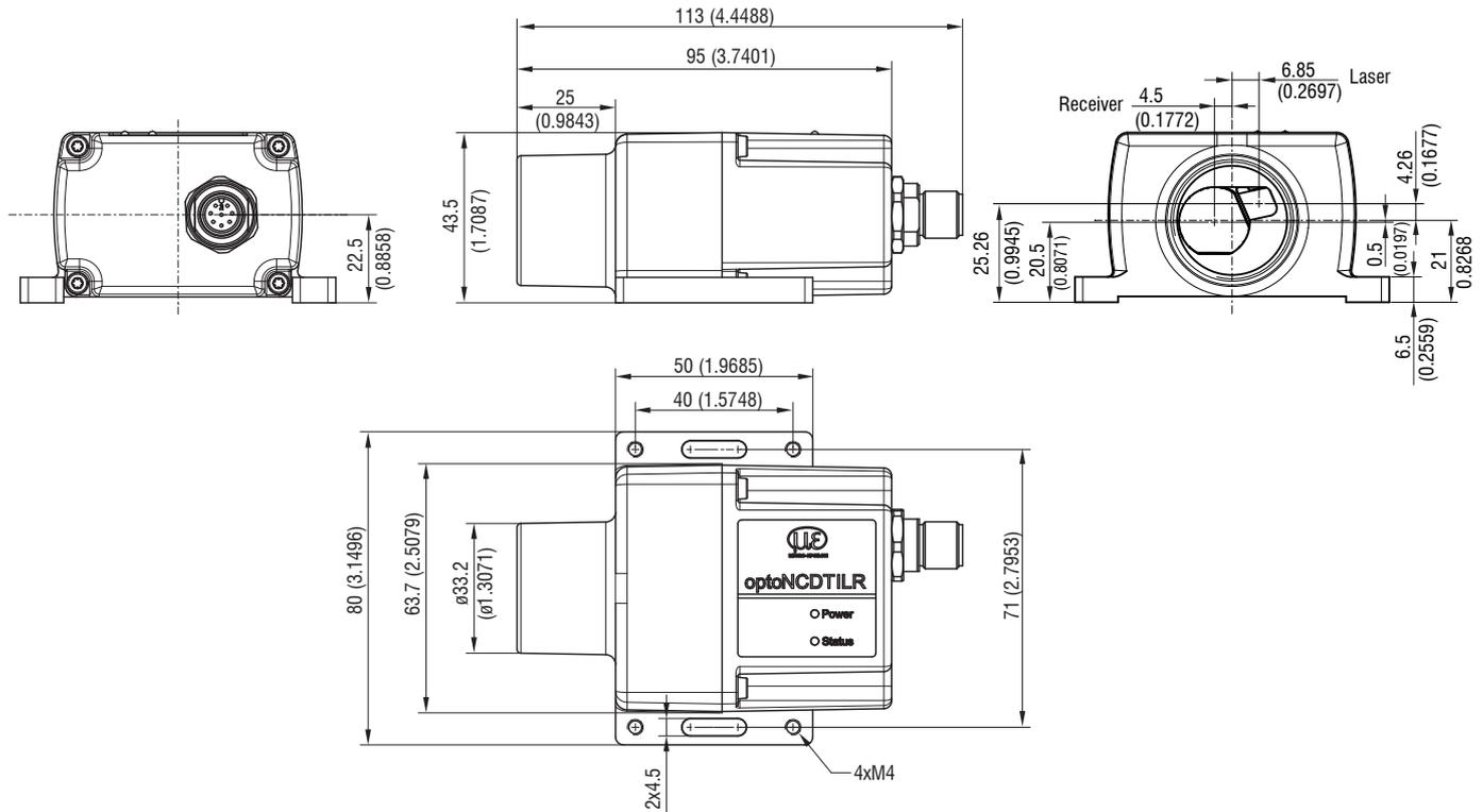
Abb. 7 Dimensional drawing optoNCDT ILR3800-100, dimensions in mm (inches, rounded off)
