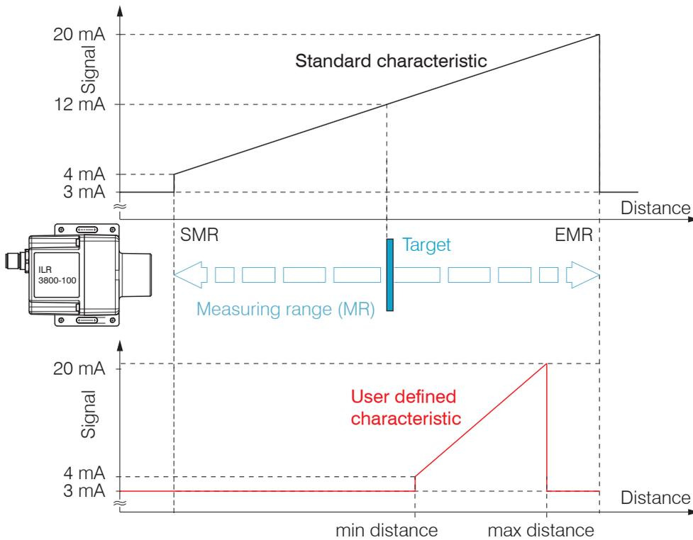
Abb. 24 Scaling the analog signal
