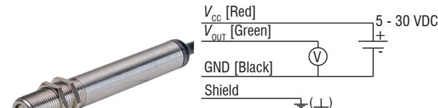
Pin assignment voltage output
